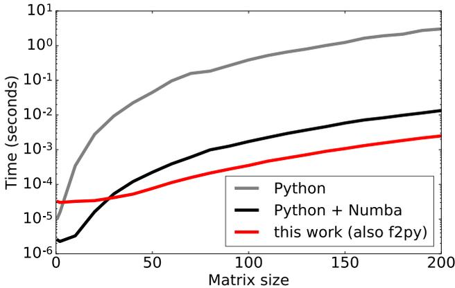
**Figure 5** Computational performance of pure Python while using our framework is the same as launching Fortran implementation through f2py.
