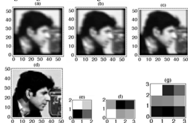
Fig. 1. (a): Test image obtained from a true image of (d) by convolving the three blurs of (e), (f), and (g). The image size is  $44 \times 45$ . (b): Image restored by removing the blur of (e). (c): Image restored by removing blurs of (e) and (f). (d): Image restored by removing blurs of (e), (f), and (g).
