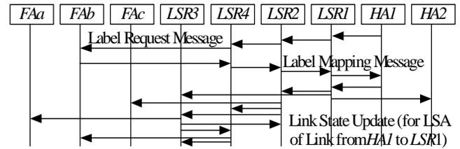
Figure 2. Sequence of establishing CR-LSP from HA1 to FAb
