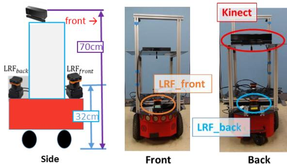
Fig.2 The guiding robot.
