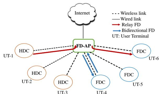
Figure 1: Structure of a full-duplex WLAN.
