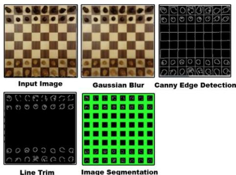
Figure 1 Process of piece existence determination
