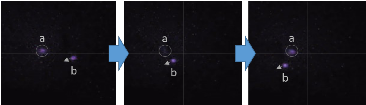
Fig. 1 Three NIR images captured by our modified webcam. Object (a) is background noise and object (b) is a retroreflective marker placed on the handle of a paring knife. The images show the movement of the paring knife from right to left, with the middle frame showing object (a) being occluded by the paring knife.
