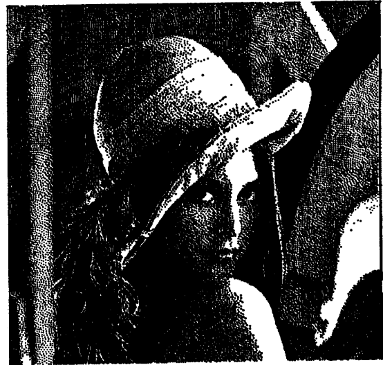
図 12 ドット径ピッチ比=2 のときの結果 (領域拡大型) Fig. 12 The result in the condition that the diameter pitch ratio=2. The reference region is extended.
