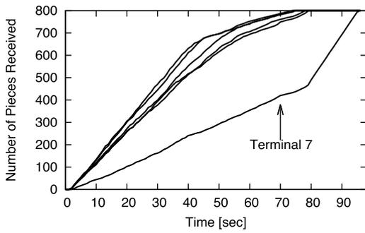
Fig. 5 Cumulative number of pieces received for each terminal (Method A, Simultaneous start).
