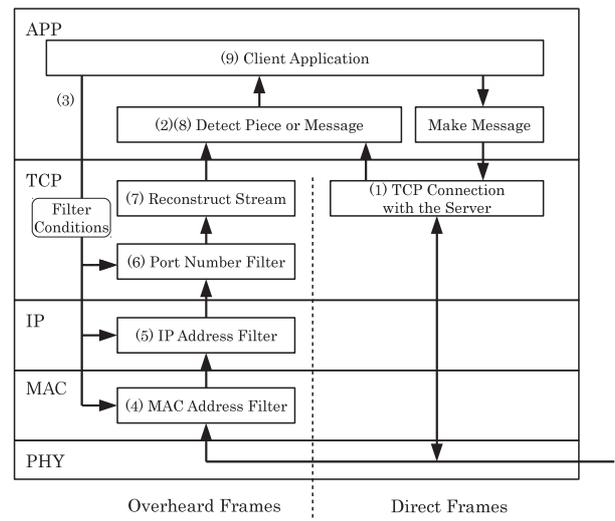
Fig. 3 Control procedures for overhearing.
