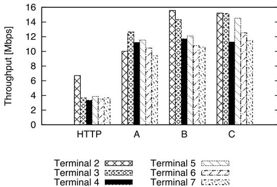
Fig. 8 Throughput of HTTP, and Method A-C (Sequential start).
