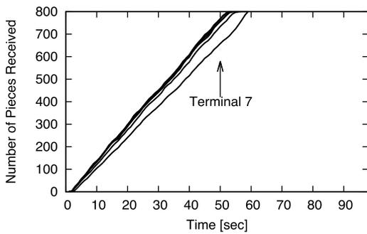
Fig. 7 Cumulative number of pieces received for each terminal (Method C, Simultaneous start).
