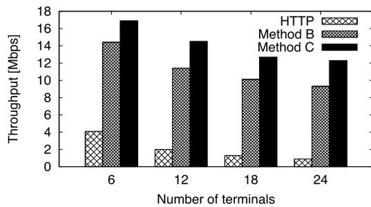
Fig. 12 Average throughput for the number of terminals (Simultaneous start).
