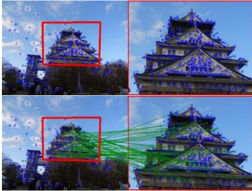
Figure 2. Top: Interest points are indicated by blue circles. Bottom: Green lines indicate matched interest points.
