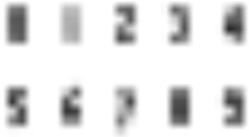
図3 低解像度化焦点ずれ劣化画像( W = 32, m_0 = n_0 = 0, r = 16 )
