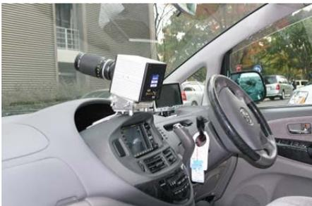
Fig. 4. High-speed camera used as receiver
