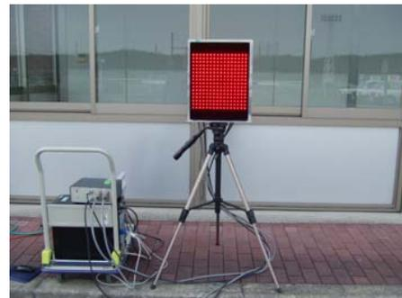
Fig. 3. LED array used as transmitter
