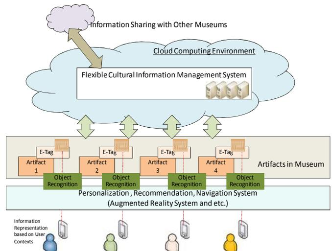
Figure 1: An Illustration of the Proposed System Architecture
