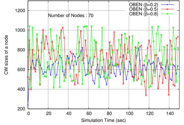
Fig. 3 CW sizes with simulation time when the  $\beta$  is changed.
