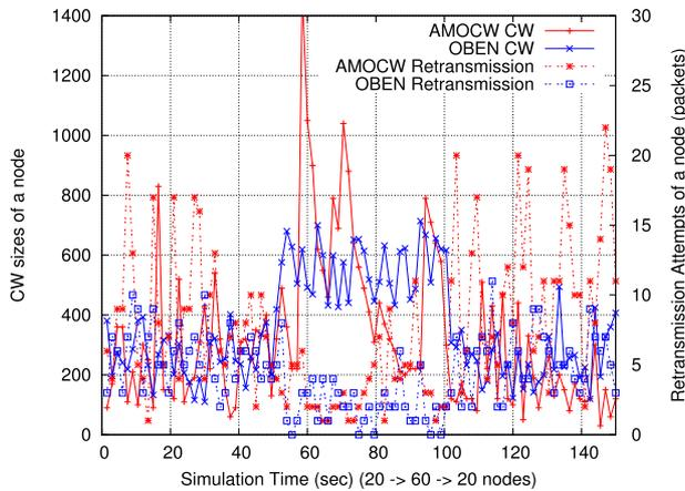
Fig. 6 CW sizes and retransmission attempts of a node with simulation time.
