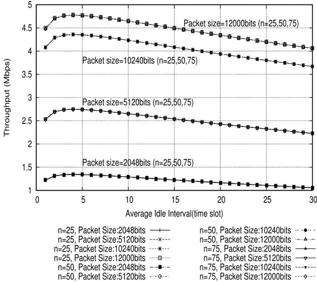
Fig. 2 Throughput with average idle slot interval.
