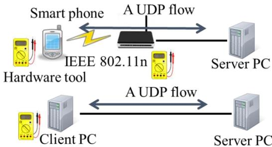
Figure 7 Experimental environments for energy consumption evaluations for smartphone and low-power compact PC
