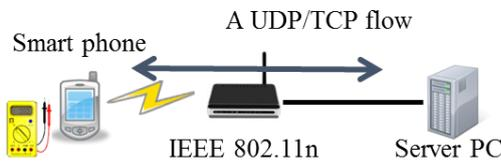
Figure 2 Experimental environment for smartphone energy consumption evaluations.
