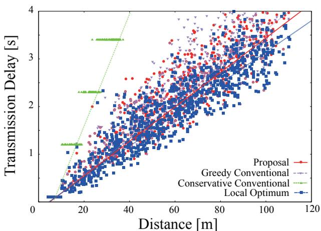
Fig. 9 End-to-End Delay in Wireless Multihop Transmissions ( 0.1 m/s ).
