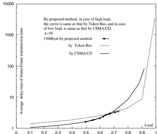
**Fig. 4** Delay characteristic of proposed method with frame length 1500 byte.
