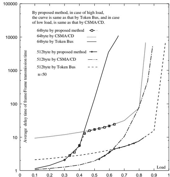
**Fig. 3** Delay characteristic of proposed method with frame length 64 byte and 512 byte.
