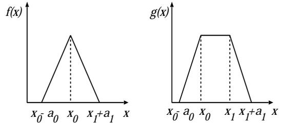
Fig. 2 Triangular and trapezoidal membership functions.
