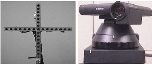
Fig. 3 Microphone array and video camera.
