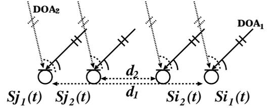
Fig. 4 DOA estimation with CSP coefficient addition method.
