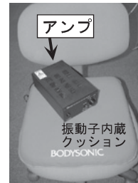
図3 Bodysonic 言語学習用システム JX-1 Fig. 3 Bodysonic JX-1 system for training of English speech/listening.
