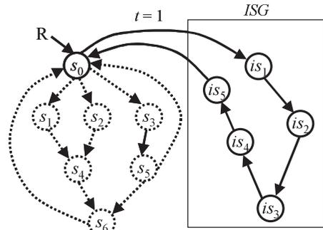
Fig. 3 Example of FSM with DFT.
