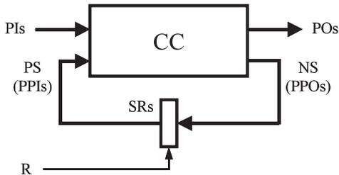
Fig. 2 Model of a synthesized sequential circuit.
