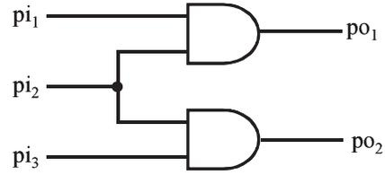
**Fig. 5** Example of a combinational circuit.
