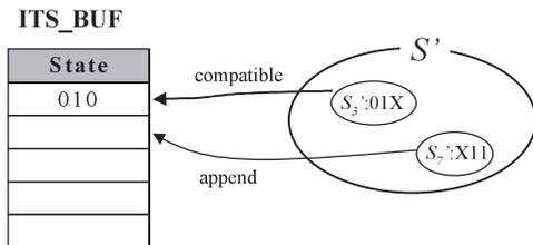
**Fig. 8** Example of invalid test state compaction buffer.
