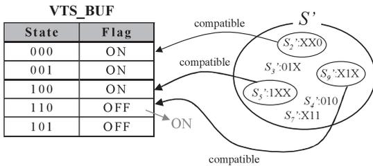
**Fig. 7** Example of valid test state compaction buffer.
