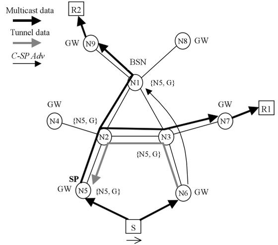
**Fig. 14** SMM-C Proc. of source handover (2): The S is moving to the access network attached to N6. The S sends *Launch* message to the new GW, i.e., N6. N6 reports to the BSN that it becomes the SP for G and sets up a tunnel to N5 through which encapsulated multicast packets are forwarded by unicasting.
