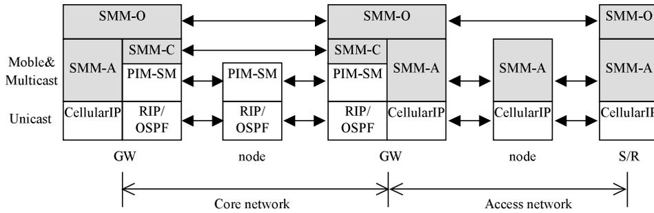
**Fig. 7** Protocol Stack: SMM consists of SMM-A, SMM-C and SMM-O. SMM-A for the access network is located on the Cellular IP and SMM-C for the core network is located on the PIM-SM.
