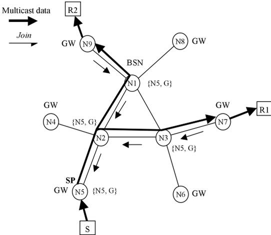
**Fig. 13** SMM-C Proc. of source handover (1): The S is sending multicast data to N5. N5 periodically informs the BSN that it is the SP for G. The BSN floods *BSM* message to all GWs. N7 and N9, which R1 and R2 belong to, send a *Join* message to N5.
