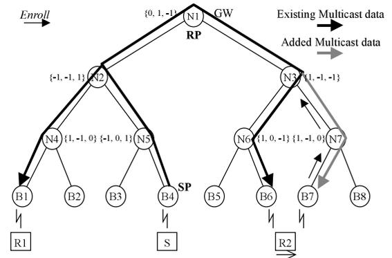
**Fig. 11** SMM-A Proc. of handover of receiving member: R2 is moving to B7 cell. R2 sends *Enroll* message to N3 via N7. N7 has no MFCE for G, then, it creates  $E_G(N7) = \{1, -1, 0\}$ . N3 already has MFCE for G, then, it update to  $E_G(N3) = \{1, -1, -1\}$ .  $E_G(N6)$  is removed by timer or *Leave* message.
