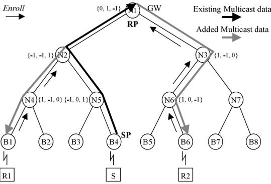
**Fig. 10** SMM-A Proc. of forming RPT and SPT (3): R1 and R2 are at B1 and B6 cells, respectively. They send *Enroll* message to N1. N4, N6 and N3 have no MFCE for G, then, they create  $E_G(N4) = \{1, -1, 0\}$ ,  $E_G(N6) = \{1, 0, -1\}$  and  $E_G(N3) = \{1, -1, 0\}$ . N2 already has MFCE for G, then, it update to  $E_G(N2) = \{-1, -1, 1\}$ .
