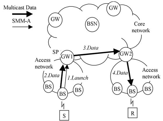
**Fig. 6** Overview of SMM Proc. 3: Upon receiving the *Page* message, the S replies to GW1 with *Launch* message to create forwarding cache entries between the S and GW1. The S starts sending multicast data, and the data are forwarded to GW1, GW2 and R.
