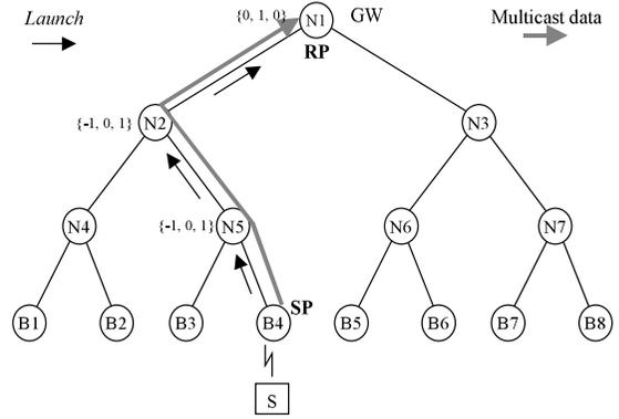
**Fig. 9** SMM-A Proc. of forming RPT and SPT (2): Now, the S is at B4 cell and sends *Launch* message to N1 to set up a path from the S to RP (N1).  $E_G(N5) = \{-1, 0, 1\}$ ,  $E_G(N2) = \{-1, 0, 1\}$  and  $E_G(N1) = \{0, 1, 0\}$  are created. Hence, constant data path is established between S and RP.
