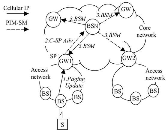
**Fig. 4** Overview of SMM Proc. 1: The S transmits its multicast group and location to GW1 using a *Paging Update* message. GW1 becomes the source point for the group and sends an *C-SP Adv* message to BSN. The BSN broadcast *BSM* messages to all GWs.
