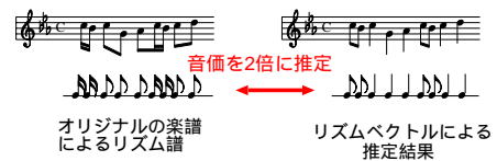
図 11 リズム譜の推定におけるテンポの多義性(正解に含める) Fig. 11 Note values are estimated as half of that of original score.
