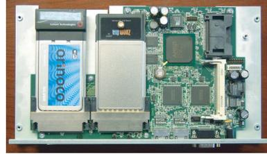
Fig. 2 Prototype SNOWNET node.
