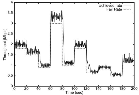
**Fig. 7** TCP throughput dynamics at sender in the case of changing number of flows.
