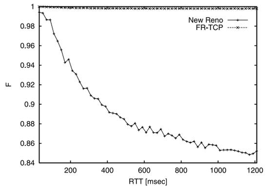
Fig. 5 Result of situation where RTT of only one flow is different from the others. It shows fairness of bandwidth against RTT is shown. RTTs of flow 1 to 5 are 40 ms and flow 6 is  $t$  ms.
