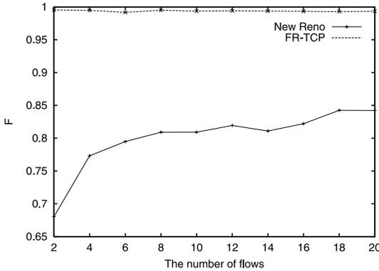
**Fig. 6** Result of situation where different number of flows are aggregated. Fairness of bandwidth against the number of flows is shown. RTTs of one half of the total flows are 40 ms and RTTs of the others are 240 ms.
