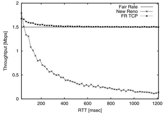
Fig. 4 Result of situation where RTT of only one flow is different from the others. It shows throughput dynamics of the flow when RTT is changing. RTTs of flow 1 to 5 are 40 ms and flow 6 is  $t$  ms.
