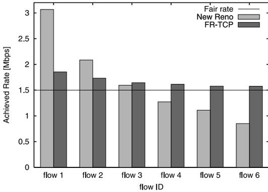
Fig. 3 Result of situation where RTTs of flow are different. Throughput of each flow is shown. RTTs of flow 1 to 6 are 40, 80, 120, 160, 200 and 240 ms.
