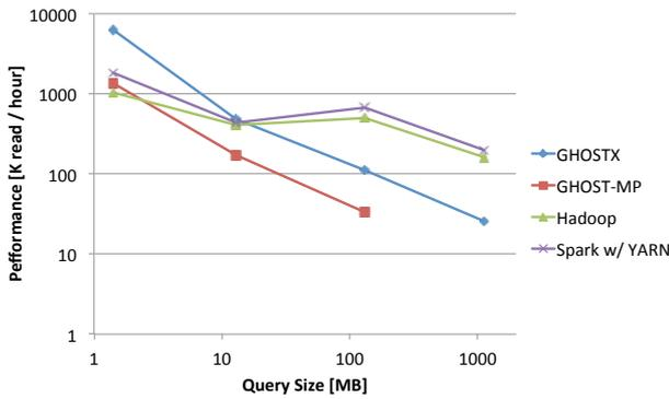
Fig. 6 Performance of data size scaling on single node
