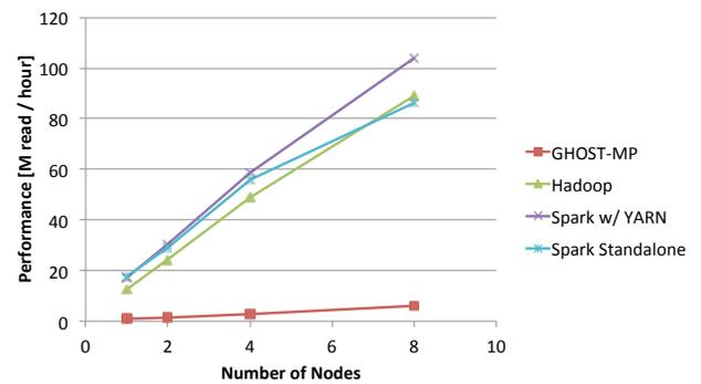
Fig. 9 Performance of weak scaling with 130MB of query per node
