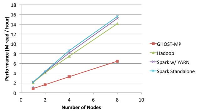
Fig. 8 Performance of weak scaling with 13MB of query per node
