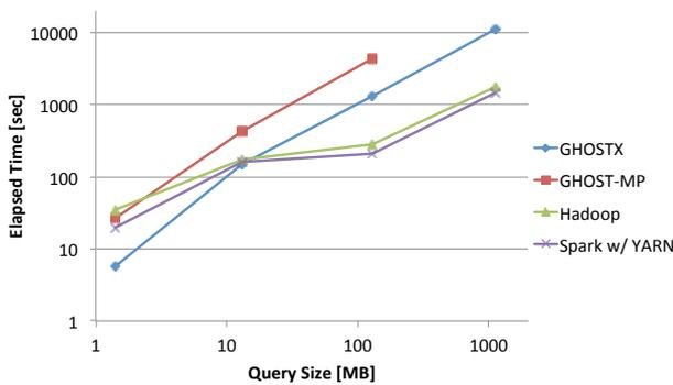
Fig. 7 Elapsed time of data size scaling on single node
