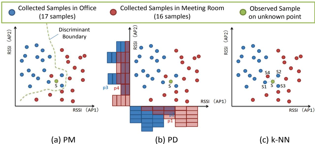
Figure 3. Room-level Localization Using Each Method
