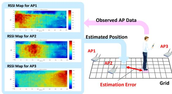
Figure 1. Wi-Fi Positioning of Fingerprint Method
