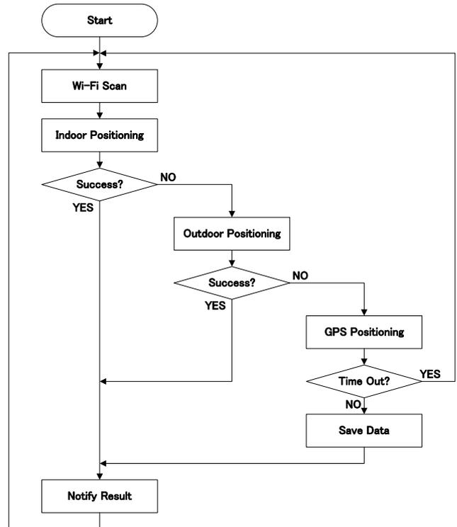
Figure 5. Flowchart of Indoor/Outdoor Seamless Positioning
