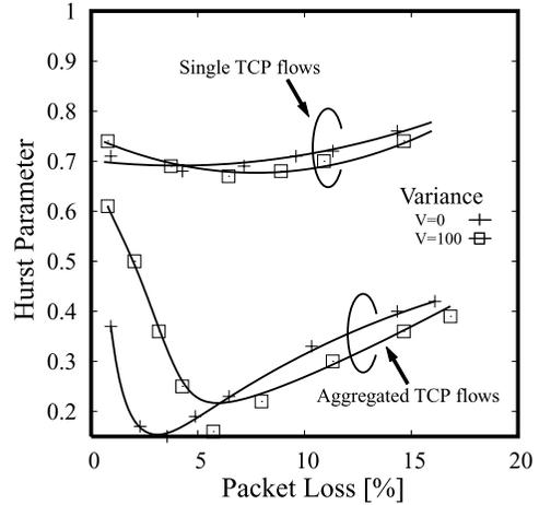
Fig. 10 Hurst parameter of aggregated and single TCP flows at different link delay variance levels.
