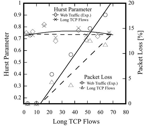
**Fig. 15** Hurst parameter and packet loss of the aggregates of the web traffic flows and the long greedy TCP flows when the web traffic is exponential distribution based.
