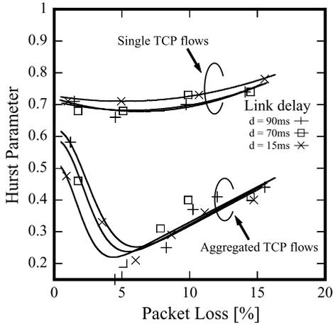
Fig. 9 Hurst parameter of aggregated and single TCP flows at different link delays.
