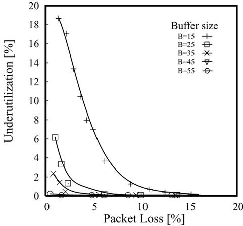
**Fig. 4** Underutilization of the bottleneck link for different buffer size values (Utilization = 100% – Underutilization).
