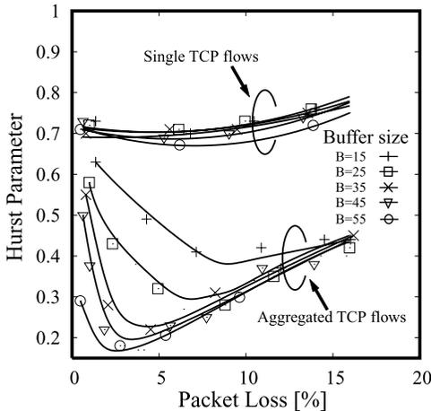
**Fig. 3** Hurst parameter of aggregated and single TCP flows at different buffer size ( $S = 3$  Mbps,  $D = 50-100$  ms).
