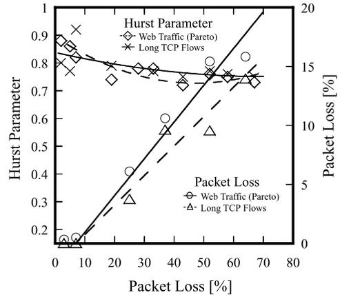
**Fig. 16** Hurst parameter and packet loss of the aggregates of the web traffic flows and the long greedy TCP flows when the web traffic is Pareto distribution based.
