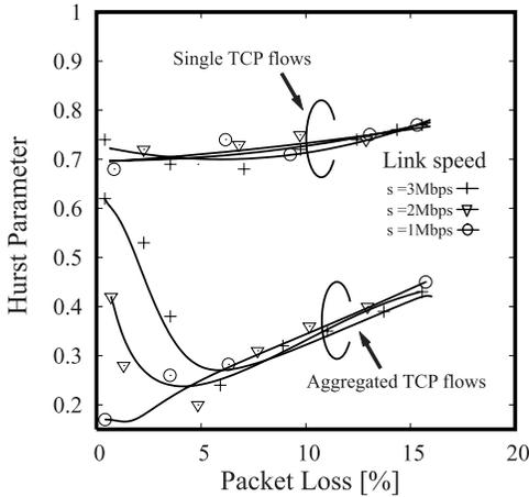
Fig. 11 Hurst parameter of aggregated and single TCP flows at different link speeds.
