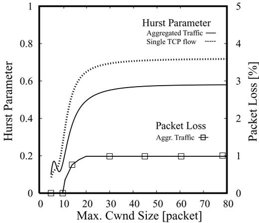
**Fig. 6** Hurst parameter of the single and aggregated TCP flows at different maximum congestion window size.
