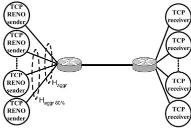
**Fig. 1** Bottleneck topology with multiple greedy TCP flows.
