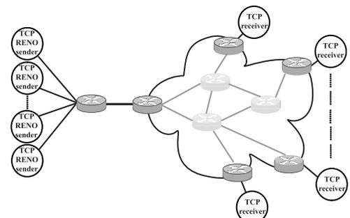
Fig. 8 Bottleneck link topology with network cloud.
