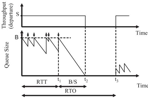
**Fig. 5** Throughput (above) and queue size (below) of the bottleneck link during synchronization.
