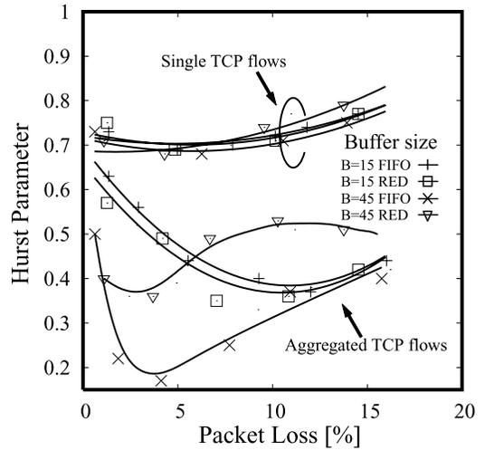
**Fig. 7** Hurst parameter of aggregated and single TCP flows at different buffer size using tail-drop FIFO and Random Early Detection schemes.
