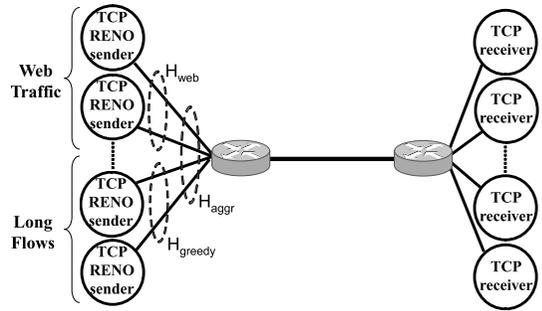
Fig. 12 Bottleneck link with web traffic and long greedy TCP flows.
