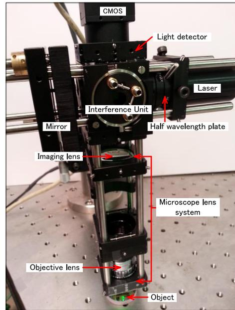
Fig. 2 Appearance of proposed 3D microscope.
