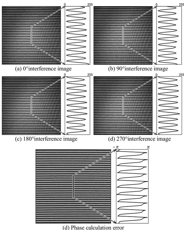
Fig. 3 Phase calculation error (object is a flat mirror).
