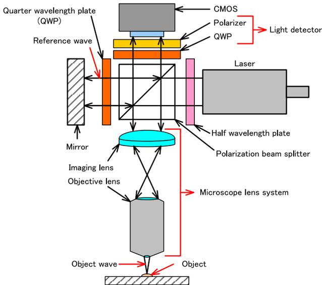
Fig. 1 Structure of proposed 3D microscope.
