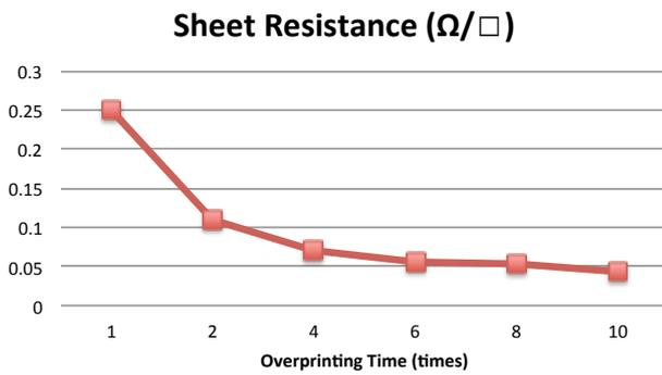
Figure 3: Change of sheet resistance depends on number of overprinting time
