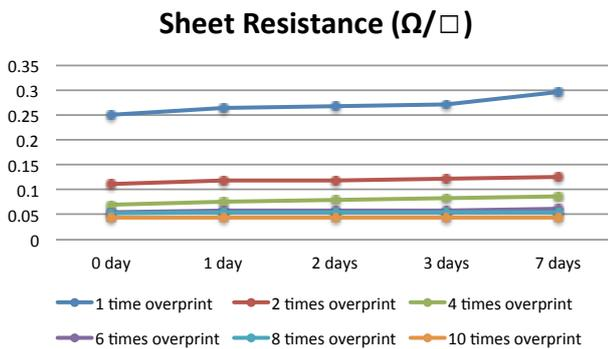
Figure 4: Change of sheet resistance after several days
