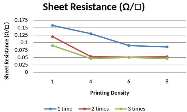
Figure 5: Change of sheet resistance depends on Density and Overprinting time
