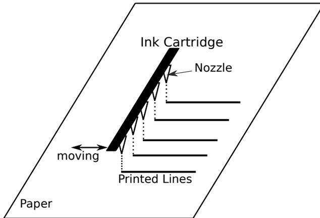
Figure 1: Inkjet printing mechanism
