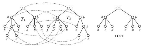
Fig. 1 Example of an LCST under the weight function giving the maximum number of nodes (i.e., f(u, v) = 1 if  $\ell(u) = \ell(v)$ , and f(u, v) = 0 otherwise) and the outdegree constraint of D = 3. The corresponding mapping M is shown by dashed curves. If D = 4, a node labeled f can be added as a child of the left child of the root of LCST.
