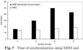
**Fig. 7** Time of synchronization using MDO and MMP peer-to-peer function.
