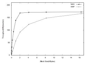
Fig. 4 Throughput comparison of strided data transfer using MDO and MMP with varying data size.
