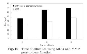
the time of MDO is almost constant even if the number of host increases. On the other, the time of MMP increases as the number of hosts increases. Especially additional communication time is required when the number of hosts is not a power of two as is the case with synchronization. And the time of MDO is up to 63% smaller than the one of peer-to-peer. From these results, we confirmed that the time for broadcast can be reduced effectively by using MDO.
