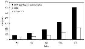
Fig. 8 Time of broadcast using MDO and MMP peer-to-peer function with varying data size.
