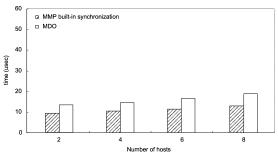
Fig. 6 Time of synchronization using MMP built-in function and MDO.
