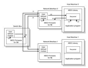
Fig. 3 Inter-process communication in MDO.
