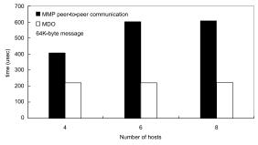
Fig. 9 Time of broadcast using MDO and MMP peerto-peer function with varying the number of hosts.
