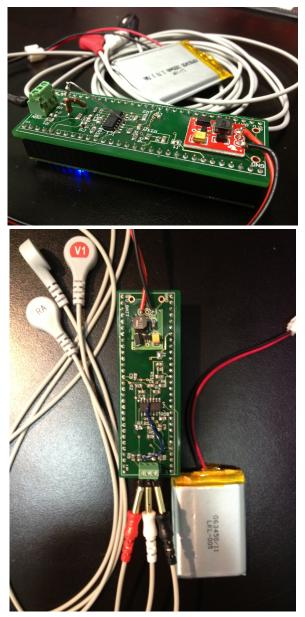
Figure 5. Wireless ECG sensor.
