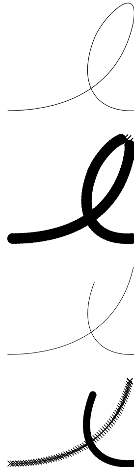
図 7 自己交差する曲線のセグメンテーションの例 Fig. 7 Examples of the segmentation of self-intersecting curves. The clustered sampling points are denoted by: solid circles the points included in the shape segment 1; crosses the points included in the shape segment 2.
