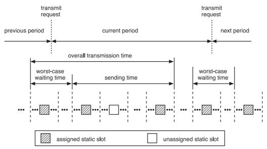
Fig. 6 Total transmission time for a communication message.
