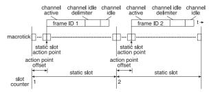
Fig. 2 Timing within a static segment.
