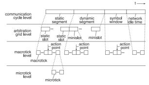
Fig. 1 Timing hierarchy within the communication cycle.
