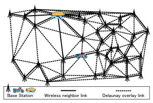
Fig. 2 Wireless mesh BSs and Delaunay overlay network.
