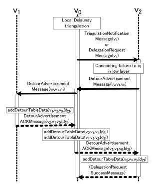
Fig. 10 Detour table construction sequence diagram.
