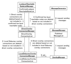
Fig. 8 Connection management mechanism based on a connection type inclusive relation.
