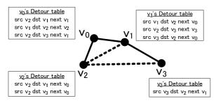
**Fig. 11** Constructing nested detour paths  $(v_3-v_1-v_2)$ .
