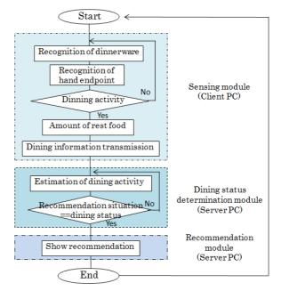
Fig. 3 System software procedures.
