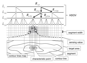
Fig. 3 Message forwarding mechanism used in HDA-RC.
