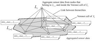
Fig. 4 Aggregation using links between hierarchies.
