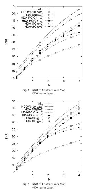
that HDA-GC (g = 0) shows higher SNR than HDA-SN when N is large. That is, we can say the HDA-GC decides the target nodes for the spatial interpolation effectively.
