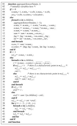
Fig. 5 Pseudocode of sensor data aggregation.
