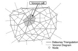
Fig. 1 Delaunay Triangulation and Voronoi Diagram.
