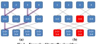
Fig.1 Example of butterfly algorithm
