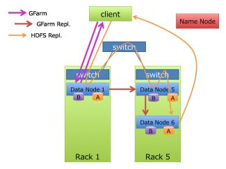
Fig. 2 Replica system on HDFS and Gfarm
