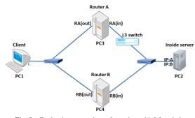
Fig. 8 Evaluation network configuration with L3 switch.
