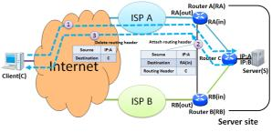
Fig. 4 Route control using the routing header.
