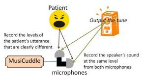
Fig. 3 Calculates the differential signals from both microphones to cancel the sounds of cadence.
