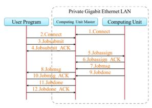
Figure 3. Protocol of standard TCP communication system
