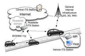
Fig. 1. ITS station reference architecture
