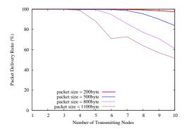
Fig. 4. Comparison between various packet sizes (bitrate = 6 Mbps, packet interval = 100 ms)
