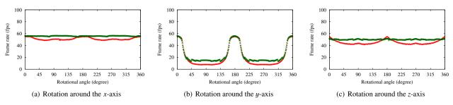
Fig. 8 Frame rates of our dynamic method and the original static method. The atom dataset was used with CUDA. Green and red plots correspond to our method and the original method, respectively.
