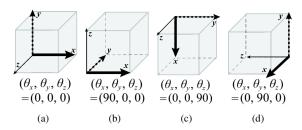
**Fig. 5** Geometrical relationship between the viewpoint and the volume axes. For simplicity, we consider here four representative viewpoints (a)–(d), which make two of the volume axes parallel to the screen axes. The *x*-axis and the *z*-axis have the smallest stride and the largest stride among the volume axes, respectively.
