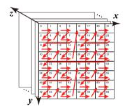
Fig. 3 Organization of a 3-D texture in CUDA. A 3-D texture consists of a bunch of 2-D slices optimized for 2-D spatial locality via Morton curve [18]. A series of red arrows represents the sequence of physical memory address in a 2-D slice. The physical address is shown in each texel's upper left corner.
