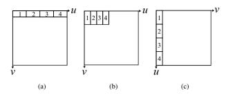
**Fig. 6** Transposed indexing of threads. (a) Horizontal TBs, (b) vertical TBs without transpose, and (c) vertical TBs with transpose. Because TB assignment is done along the *u*-axis in a cyclic manner, (b) a naive assignment of vertical TBs is not symmetric to (a) that of horizontal TBs. In contrast, our transposed indexing exchanges the *u*- and *v*-axes so that its assignment is symmetric to (a).
