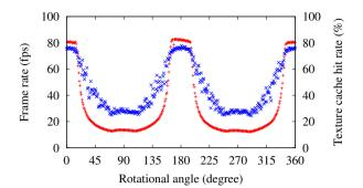
Fig. 2 Relationship between the frame rate and the hit rate of texture cache. These results were obtained with a fullerene dataset. The horizontal axis represents the rotational angle around the *y*-axis. Red and blue lines show the frame rate and the hit rate, respectively.
