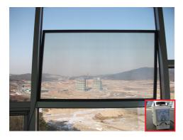
Figure 2. See-through window display with voltage regulation
