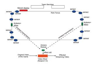
Figure 2. Layout of devices around the rink and video control flow
