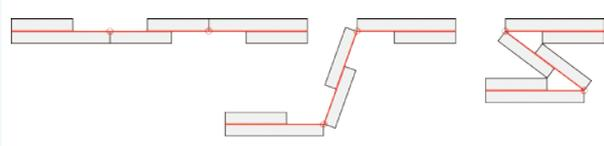
図-20 厚みのあるパネルで機構を作る<sup>6)</sup>
