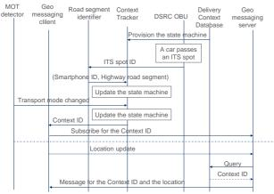
Fig.5 Sequence diagram of alternative 2
