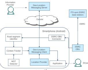
Fig. 7 Prototype of the 2<sup>nd</sup> architecture alternative.
