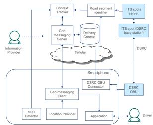
Fig. 2 Solution architecture alternative 1.
