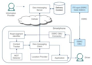
Fig. 3 Solution architecture alternative 2.
