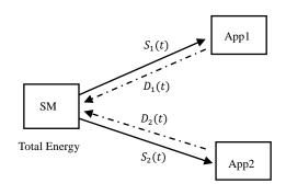
Fig. 3: Modelling structure for SM and Home Appliance
